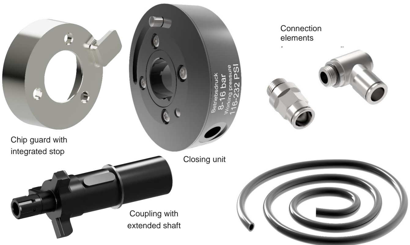
Figure 6: Assemblies of the coolant-operated closing device
