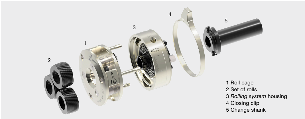
Fig. 4: The five subassemblies of the rolling system
